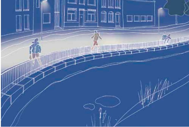
- Optic LensoFlex2® “Narrow road” 5098 - For S classification according to CIE 115
