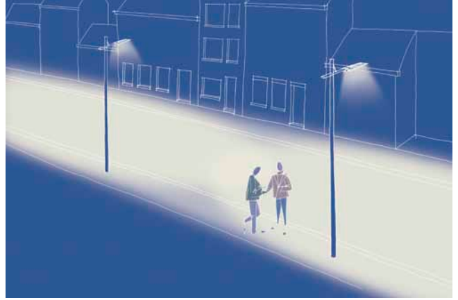
- Optic LensoFlex2® “Residential street” 5093 - For M4 classification according to CIE 115 - SR > 50% included
